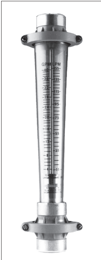
Fig. 6.36 A commercial rotameter. The float rises in the tapered tube to an equilibrium position, which is a measure of the fluid flow rate. (Courtesy of Blue White Industries, Huntington Beach, CA.)
